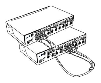
Figure 2. Cascade Configuration
